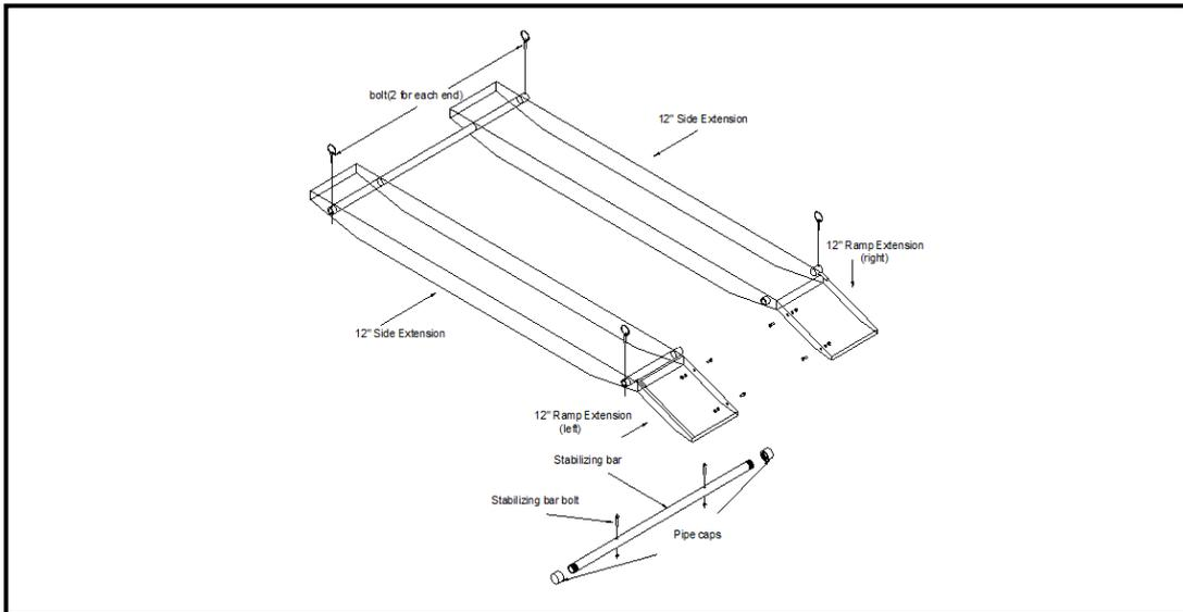
1. Insert pipes from extension panel package through holes in lift table.
