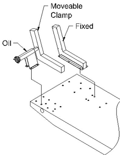
Align two inside hole of the fixed clamp over the existing vise hole pattern as show.
